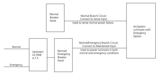
The sense input is used to detect whether normal utility power has been lost. This will force the luminaire on at 100% intensity running from the maintained supply. There is no control of the luminaire via wireless- or wired-DMX until normal utility power is restored to the sense input.
