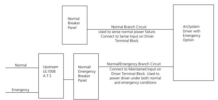
If normal power to the sense input is lost, the driver will force the luminaire on at 100% overriding all other control signals. There is no control of the driver/luminaire via wireless ArcMesh or wired DMX until normal power is restored at the sense input.
